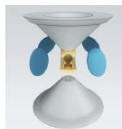
A schematic of the Super-X™ geometry including 4 SDD detectors arranged symmetrically around the sample and the objective lens pole pieces. This schematic is not to scale.
