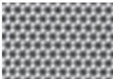
HAADF STEM image of a graphene lattice imaged at 80kV.
