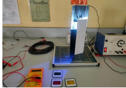
Figure 2.1: Project simulation by using RGB led with blue filter
