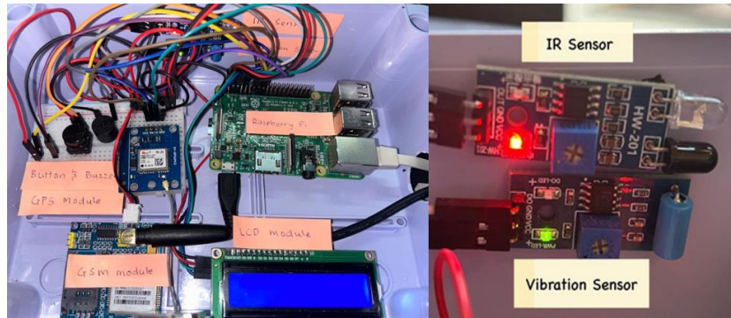
Figure 2 : View of the Used IoT Components
